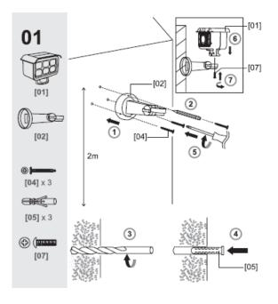
Using the adjustment screw on the side of the wall mount bracket, adjust the angle of the light as required and tighten to secure in the desired position.
